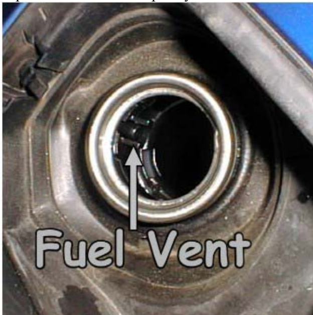
Topping up using the vent valve
